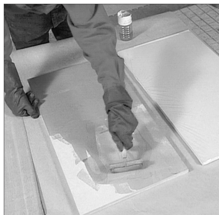
Figure 2. To glue 1/32 " veneer to a substrate, spread glue only on the substrate.
