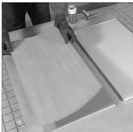
Figure 3. With glue applied, carefully place the veneer on the substrate.
