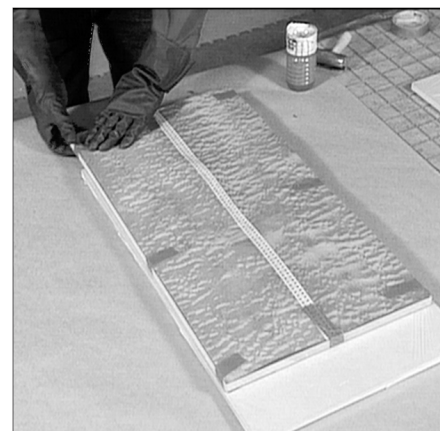
Figure 4. With veneer attached to both sides, tape the "wood/glue" sandwich.
